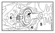
Squeeze grease into the gearbox housing (arrow) between the cam (4) and cutting blade (5) a little at a time (max. 5 g (1/5 oz)) while turning the drive pinion (6) with a hex key to distribute the grease evenly – avoid contact with the cutting blades.
