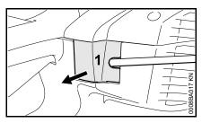
Carefully pry open the flap (1) with a suitable tool (e.g. combination wrench).
