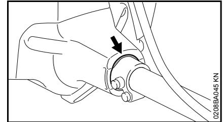
A vibration-absorbing rubber element is installed between the powerhead and the shaft. Have it checked in the event of noticeable wear or constantly increased vibration.
