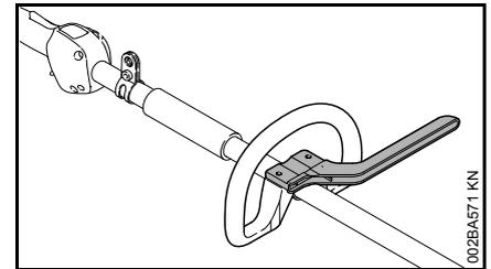
A barrier bar may have to be mounted to suit the tool you intend to use – see "Approved Combinations of Cutting Attachment, Deflector, Handle and Harness".
