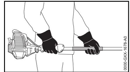
Right hand on control handle, left hand on handle hose on drive tube, even if you are left-handed. Wrap fingers and thumbs firmly around the handles.
