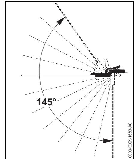
The angle of the cutter bar can be adjusted upwards in 4 stages from 0° (straight) to 55°, and downwards in 7 stages from 0° to 90° (right angle facing down). There are therefore 12 possible working positions.
