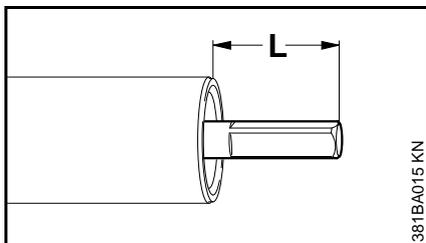
The drive shaft must not project from the tube more than  $L = 22 \text{ mm}$  (7/8 in).
