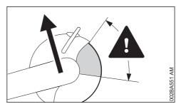
Kickback occurs when the cut-off machine is suddenly thrown up and back in an uncontrolled arc towards the operator.
