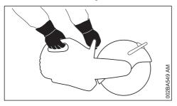
Always hold the machine **firmly with both hands**: Right hand on the rear handle – even if you are left-handed. To ensure safe control, wrap your fingers tightly around both handles.
