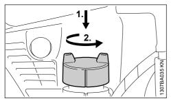
Press the filler cap down as far as possible by hand, then turn it counterclockwise (approx. 1/8 turn) and remove
