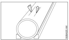
Use wedges and/or leave ridges that are broken after cutting
