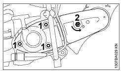
Prior to tensioning of the ribbed V-belt, the nuts (1) must be loosened and the arrow on the tensioning nut (2) must point to **0**.
