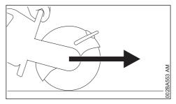
The cut-off machine pulls forward, away from the user, when the abrasive wheel touches the object to be cut from above.
