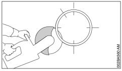
Always start at the bottom, use the upper quarter of the abrasive wheel for cutting
