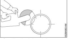
Second lateral cut in the marked area – never cut into the area of the last cut, to ensure a firm hold on the part of pipe to be cut
