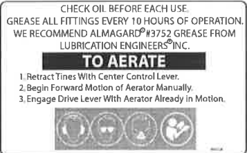
Fig. 4 LABEL AERATING INST PL
