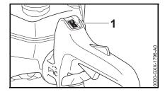
The stop switch (1) is in the normal run position I.
