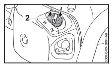
Depress the outer ring (arrows) of the choke knob (2) and then turn it to <u>∠</u>.
